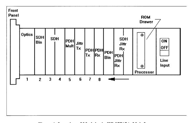
Figure 1 Location of Modules in HP 37717A Mainframe
